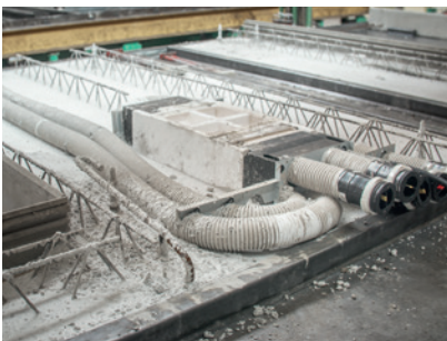
The bare brickwork set is integrated in the prefabricated wall in the factory
